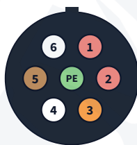
Round 6 pin + PE, applicator end
